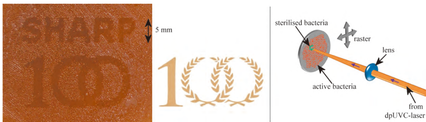
Fig. 4 A demonstration of sterilisation of bacteria using the dpUVC-laser. The dpUVC-laser beam was rastered to sterilise the surface in the pattern of a "SHARP 100" logo. The pale spots are bacterial growth; the dark brown area of the logo was sterilised. The diagram on the right shows the sterilisation setup.
