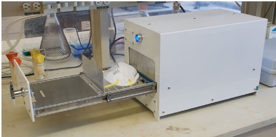
Figure 6. Prototype of a low-cost “Local UV” box for decontamination of N95 masks. The box is shown with the drawer fully opened and an N95 mask placed on the quartz support rods.
